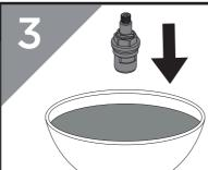
Place cartridges in a suitable solution and soak until fully de-scaled.
