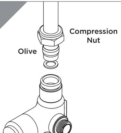
Push the short connecting tube into the top outlet on the shower valve (not supplied) ensuring the nut and olive are fitted to the connecting tube.
