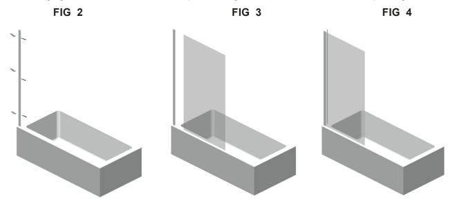
5. Seal the join between the wall profile and wall on the outside and 50mm vertically between the wall profile and the glass.
