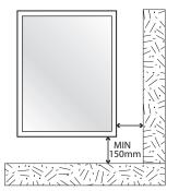
The product must be installed with a minimum distance of 150mm between the infrared sensor and any adjacent obstruction to ensure correct function of the sensor (see diagram).
