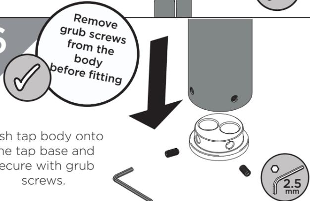
Remove grub screws from the body before fitting
