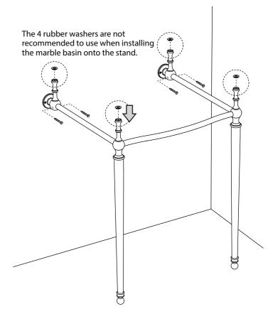
For ceramic basin, place the basin in position ensuring that it is level. The basin must be fixed to the wall at the rear using appropriate wall fixing screws.
