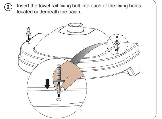
Pull the fixing bolt up so that it catches on the inner surface of the basin, and then tighten, but only tight enough to prevent the fitting sliding too much.
