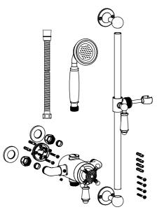
Step 1: Make sure all the components above are complete. Assemble shower holder to sliding rail.
