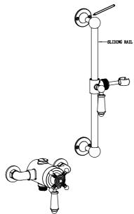
Step 5: Place the sliding rail against the wall in a proper position and make markings.
