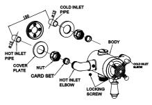
Step4: Place the components and body as per the order above. Turn nuts on the body, then fix the mixer onto the wall with locking screws, tighten the nuts with spanner to seal.
