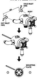
Step 2: Place the body on the wall and make markings. Then remove the body, place the mounting plate in the center of the marking, mark 4 locating holes.
