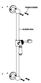
Step7: Fix the top and bottom brackets of the sliding rail with screws.
