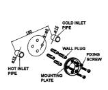
Step3: Drill four holes of Ø8mm with depth of 45mm,tap in wall plugs.Then fix the mouting plate onto the wall with screws.
