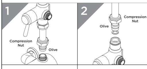
Push the short connecting tube into the top outlet on the shower valve (not supplied) ensuring the nut and olive are fitted to the connecting tube. Tighten the nut fully using a suitable spanner to ensure a water tight seal.
