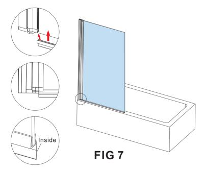
6.Insert the screen into the wall profile. Ensure the bottom seal on the moving panel A is parallel to the top surface of the bath.
