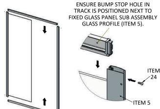
SLIDE THE TOP & BOTTOM TRACKS INTO THE GLASS PROFILE AND MAGNETIC PROFILE UNTIL FLUSH.
