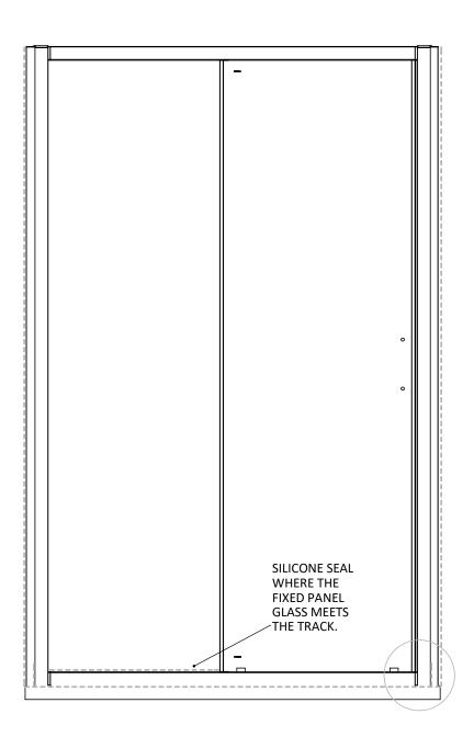
EXTERNALLY SILICONE SEAL THE WALL PROFILES WHERE THEY MEET THE WALL AND THE BOTTOM PROFILE WHERE IT MEETS THE TRAY. ALL IN A CONTINUOUS BEAD.
