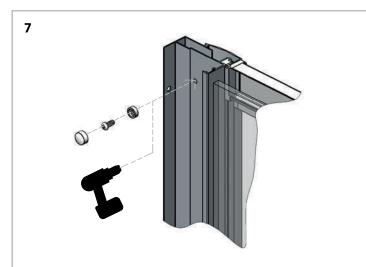
WHEN THE FRAME IS READY TO BE FIXED, DRILL THROUGH THE HOLES IN ITEMS 2 & 5 WITH A 3mm DRILL BIT.
