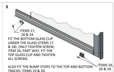
DO NOT OVERTIGHTEN THE SCREWS. OTHERWISE IT WILL SHOW THROUGH ON THE FRONT FACE OF THE TRACK.
