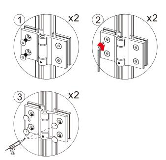
Before final tightening of the hinge screws make sure the 2nd glass panel is pushed towards the first panel
